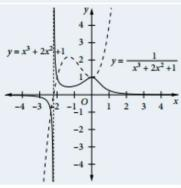
As the Examples above show, a maximum turning point on the original function becomes a minimum turning point on the reciprocal function (or equivalent asymptote). A minimum turning point on the original function becomes a maximum turning point on the reciprocal function (or equivalent asymptote).
