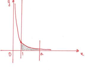
$$V = \pi \int_{A}^{\alpha} x^{-2} dx = \pi \left[ \frac{x^{-1}}{-1} \right]_{1}^{\alpha} = \pi \left[ -\frac{1}{x} \right]_{1}^{\alpha}$$
