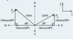
$$\begin{split} \underline{F}_1 &= 120\cos 30^{\circ} \underline{i} + 120\sin 30^{\circ} \underline{j} \\ &= 103.92 \underline{i} + 60.00 \underline{j} \\ \underline{F} &= \underline{F}_1 + \underline{F}_2 \\ &= 103.92 \underline{i} + 60.00 \underline{j} - 114.91 \underline{i} + 96.42 \underline{j} \\ &= (103.92 - 114.91) \underline{i} + (60.00 + 96.42) \underline{j} \\ &= -10.98 \underline{i} + 156.42 \underline{j} \end{split}$$
