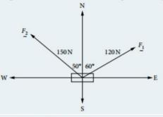
Resolving forces into horizontal  $(\underline{i})$  and vertical  $(\underline{j})$  components:
