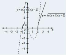
The graph of  $y^2 = x(x+1)(x-2)$  is undefined for x < -1, 1 < x < 2. The graphs meet at (-1, 0), (0, 0), (2, 0).
