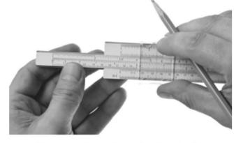
logarithms and devices called 'slide rules' (see the picture at right) were used to perform calculations involving multiplication, division and corresponding operations, e.g. raising to a power or finding the square root. The slide rule had a logarithmic scale and used the fact that you can find the product of two numbers by adding their indices or logarithms.
